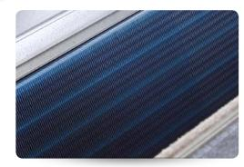
All models in the HTU range feature evaporating coils with hydrophilic coating. This special coating - together with an adequate adjustment of air throughflow speeds - helps condensate collection during the dehumidification process, avoiding dripping on the inside and outside of the unit.
